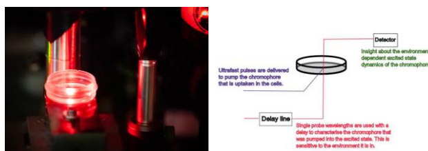
Fig: in cellulo transient absorption setup and a schematic figure of the setup
